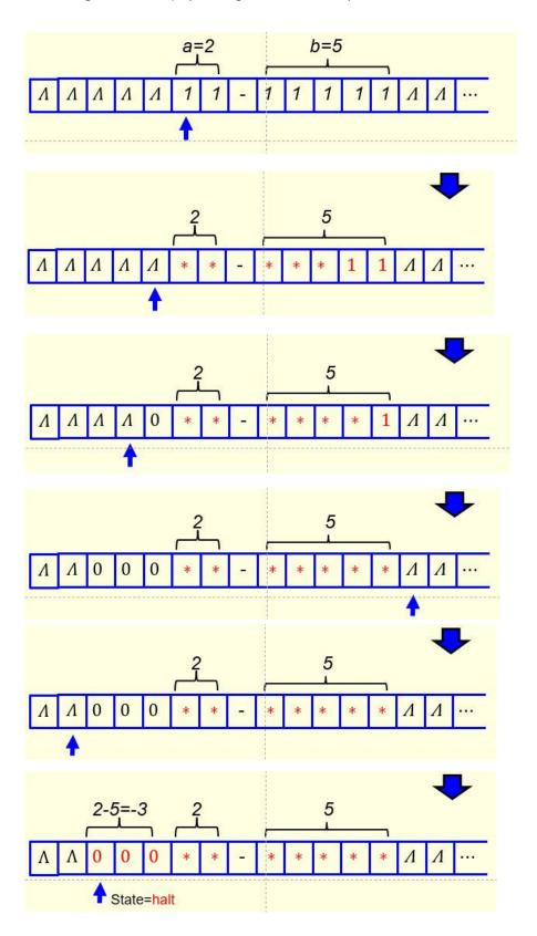
Your task here is to fill out the three blanks in the following figure to make it a TM that can subtract a bigger number from a smaller number as well.
