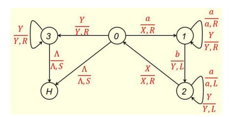
One can extends the concept of this TM to design a new TM to accept the language  $\{a^nb^nc^n\mid n\in N\}$ . The new TM has 14 distinct instructions and 6 states: 0, 1, 2, 3, 4, and halt. It uses two implicit stacks to match the number of a's in the string with the number of b's and the number of c's in the string.
