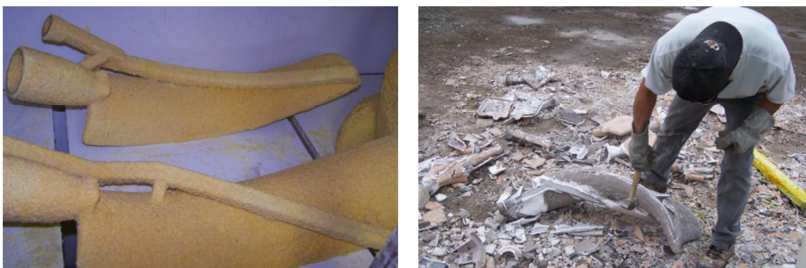
Fig. 12. (a) Slurry shell around wax copies; (b) removing the plaster shell after the casting process.
