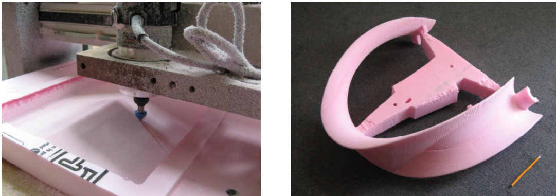
Fig. 10. (a) The NC milling machine used to produce master patterns; (b) the smaller master segment obtained by NC milling.
