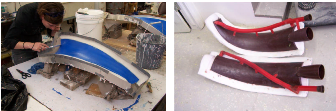
Fig. 11. (a) One third of the larger master segment used to form a mold; (b) wax copy of this sub-segment with sprues and funnels.
