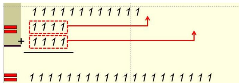
The TM looks like as follows. The portion circled by the red dotted curve is to perform the addition job (putting a copy of  $m$  1's at the end of  $n$ ) and the portion circled by the blue dotted curve is the portion that does the counting (making sure  $n$  copies of  $m$  in unary form are put at the end of  $n$ ).
